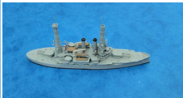
In 1908 USS Mississippi introduced the lattice cage mast as a robust means of supporting fire control equipment. A second mast was fitted in 1911 as depicted in this Navis model
